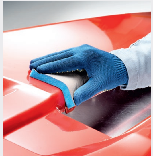
Manual sanding of hard-to-reach areas e.g. keying/sanding of plastic parts, intermediate sanding in hard-to-reach areas
