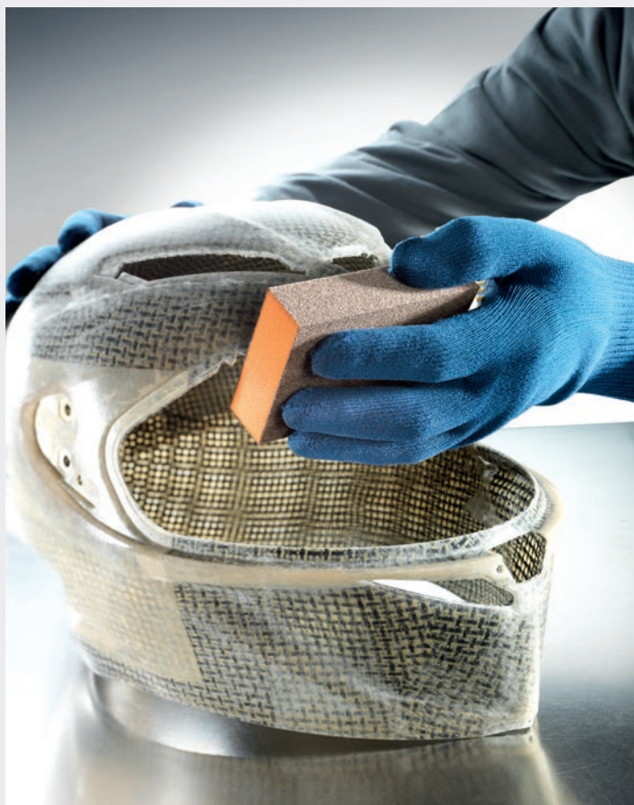
Manual sanding of special shapes and contours e.g. preparation for painting over composites
